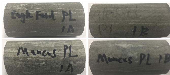
Fig. 1 —Two Eagle Ford shale core plugs (top row) and two Mancos shale core plugs (bottom row) for the PDP permeability measurements. The shale core plugs were 2 in. in length and 1 in. in diameter. The shale bedding plane direction was parallel to the core plug axis direction.
