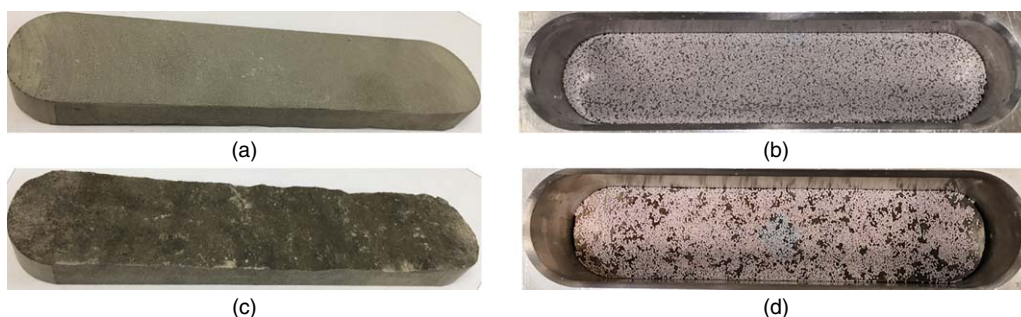
Fig. 9—Eagle Ford Shale plates having (a) smooth rock surface and (b) rough rock surface, and proppant placements on the plates having (c) smooth rock surface and (d) rough rock surface in the fracture conductivity cell.
