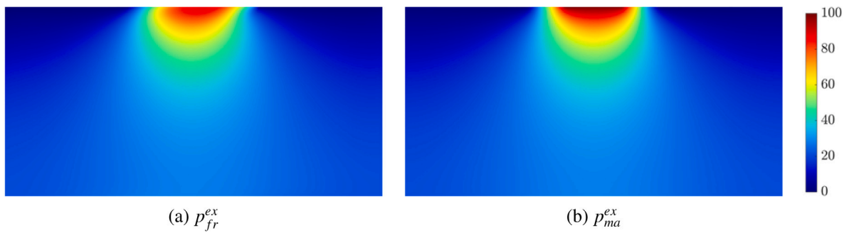
Fig. 10. Spatial variation of excess fluid pressure at t = 0.1 h for an elastic porous medium, kPa.
